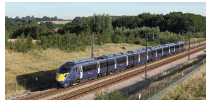
Japan-made trains operate on the new high-speed line connecting London to the Channel Tunnel. The trains can run freely on both conventional lines and dedicated high-speed lines.
