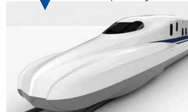
The front shape of the N700S has been evolved to cut noise and wobble for a more comfortable ride.
