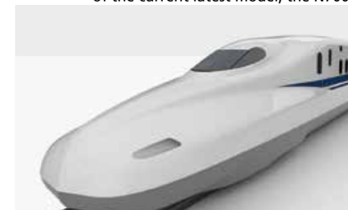
Newly developed "Dual Supreme Wing" of the N700S
